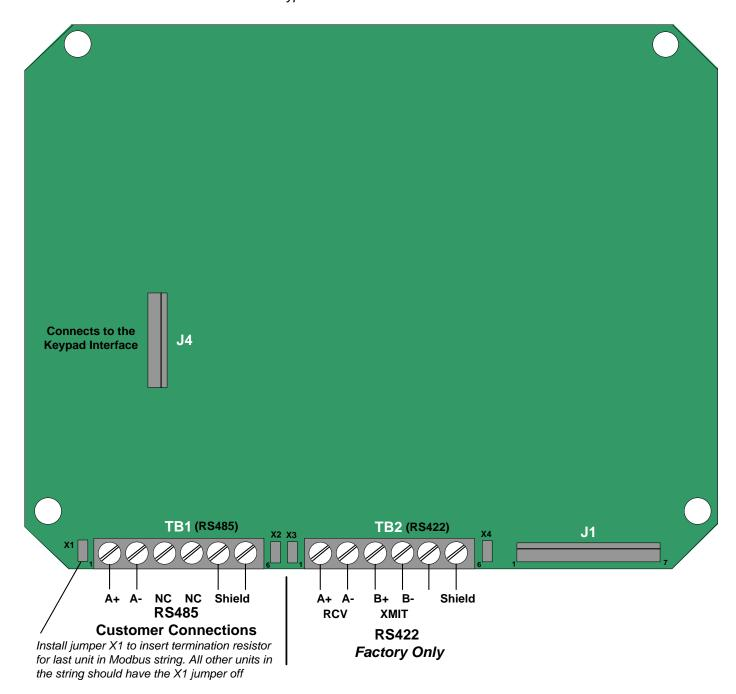
FIG. 2.9d RS485 / RS422 Communications Board
