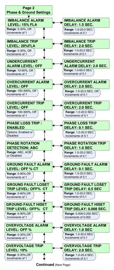
**SP3.6 Phase Loss Trip**: When enabled, the Soft Starter will trip the motor off-line upon a loss of phase power.
