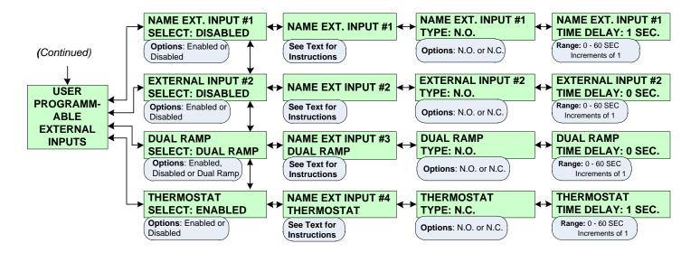
**SP6.5 User Programmable External Inputs**: The controller provides up to 4 digital external inputs which are individually programmable. A description name can be assigned to each individual input for easy identification.
