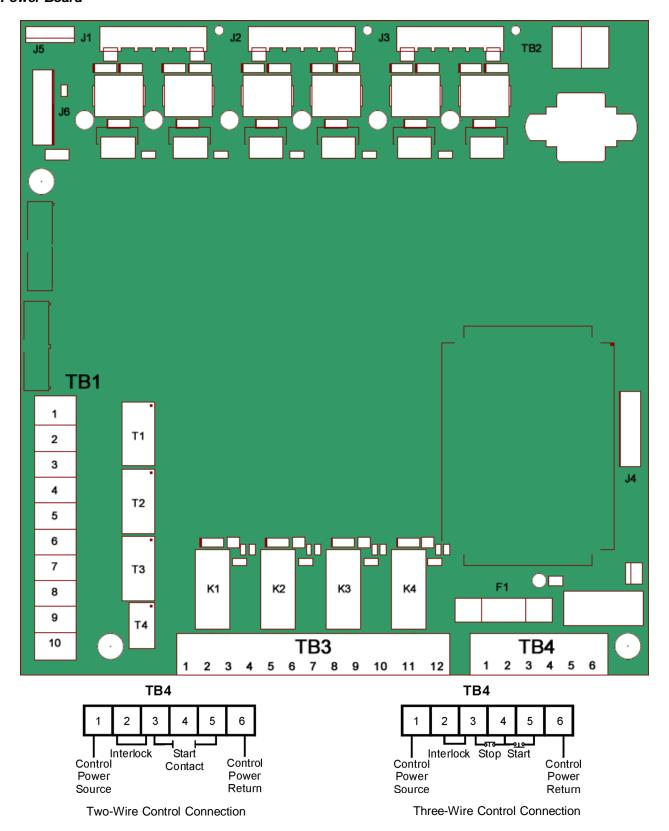
Relay Contacts on Power Board Rated 240 VAC, 5A, 1200VA
