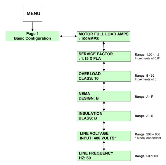
**SP1.1 Motor Full Load Amps (FLA):** Allows the user to enter the motor's FLA rating. Range of adjustment is 50 - 100% of units maximum current rating (described below).
